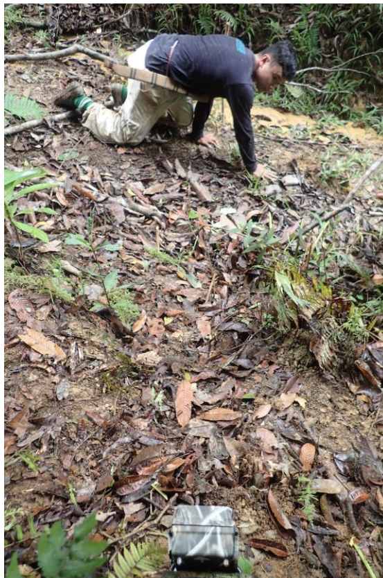
Crawl test before initiate the actual session of camera trapping to make sure the camera captures the perfect images of the animals
